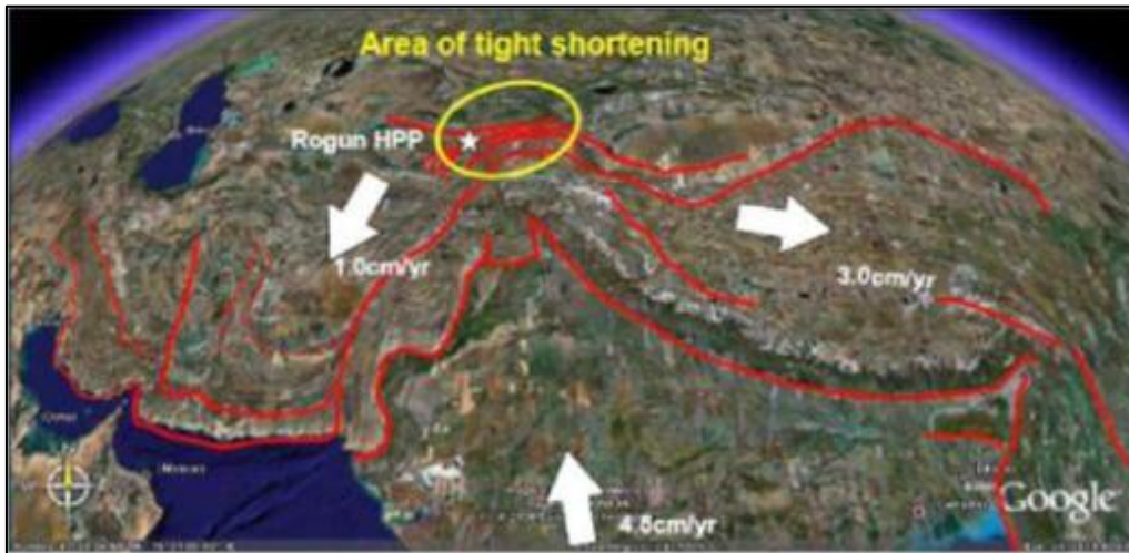
Figure 5: India-Asia collision and induced deformation within Eurasia. Rogun HPP is located within the western syntax of the Himalaya, characterized by intensive shortening.
