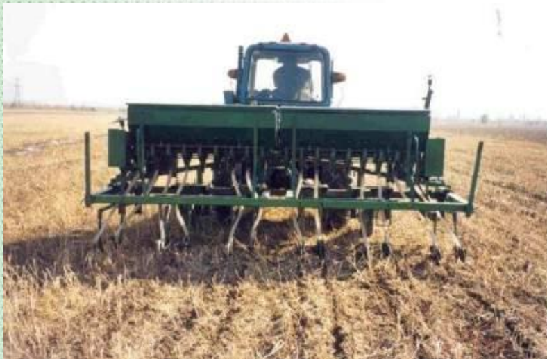
Locally developed direct seeder for bed-planting
