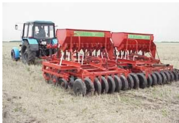
The local seeder SZS-2,1 with the Brazilian disk furrow openers and cutting discs
