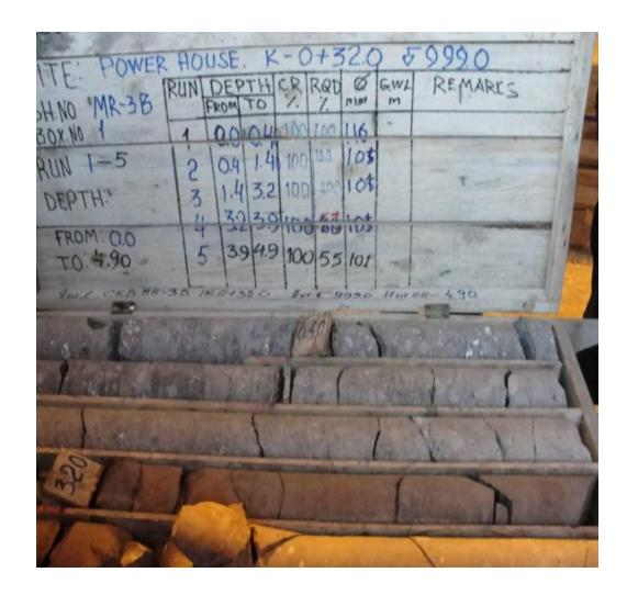
*Cores of siltstone behind the concrete lining at +999.*
