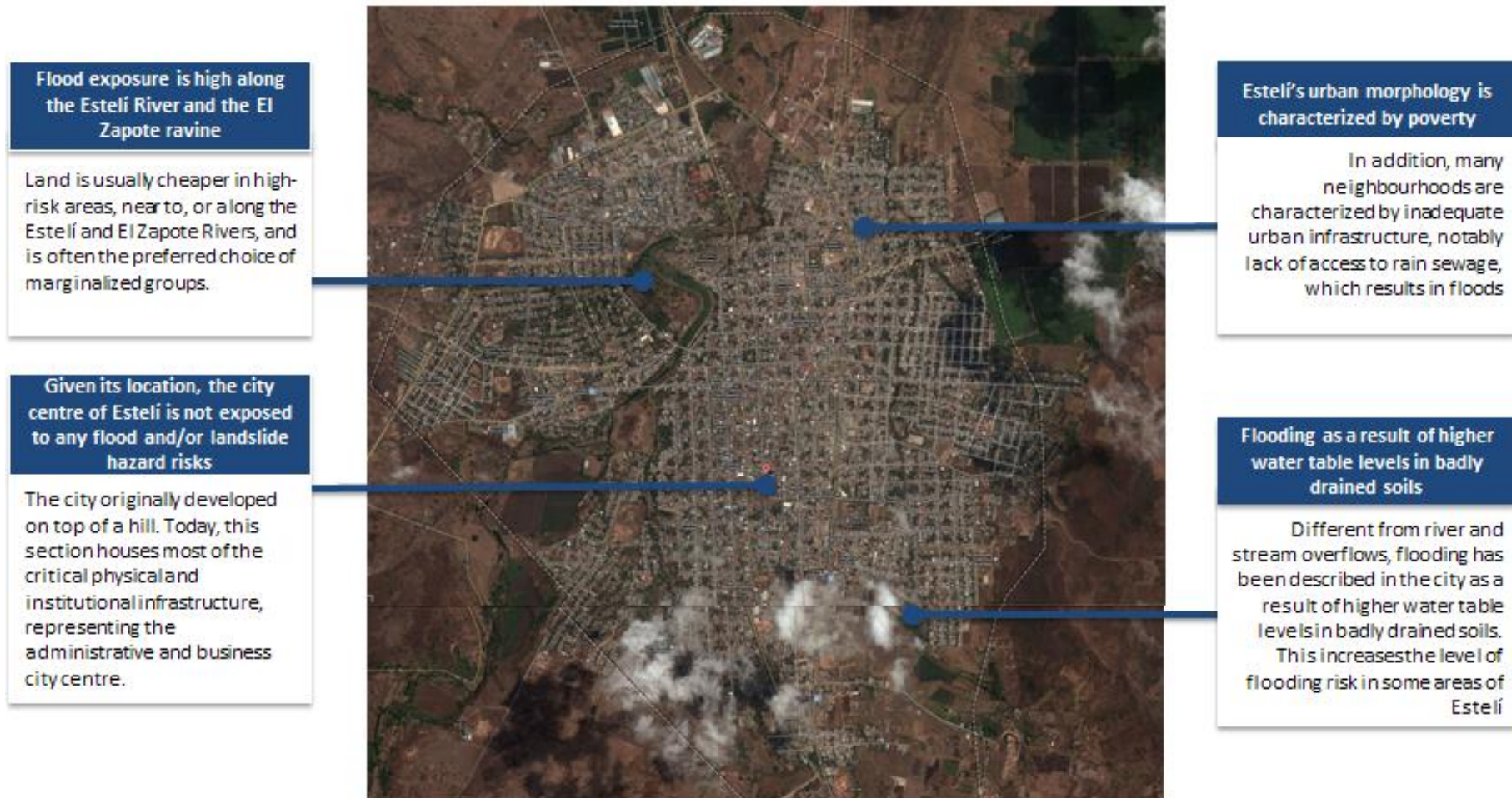
Figure 5.1 Predominant features of the built environment in Estelí that impact upon flood and landslide hazard risks.
